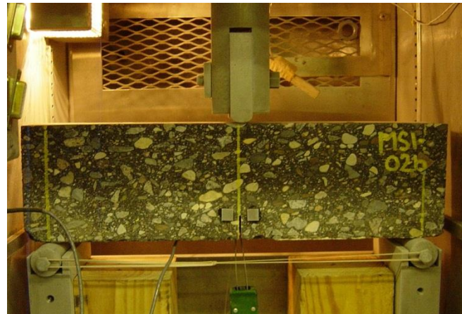
Figure 50. Single Edge Notched Beam (SENB) testing configuration (Braham).
