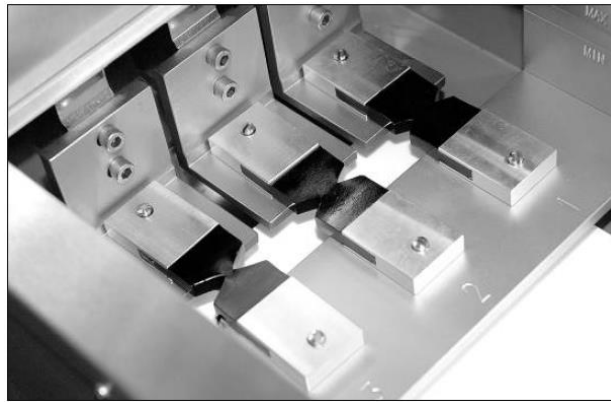
Figure 4. DENT test specimens in ductiliometer (Gibson et al., 2012)..
